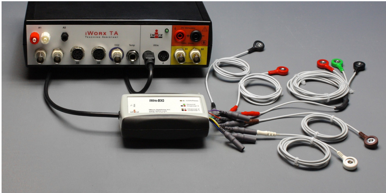
Figure HH-7-S4: iWire-B3G cable with C-ECG-IE indifferent electrode cable attached to an IXTA for recording a limb and a chest lead ECG.
